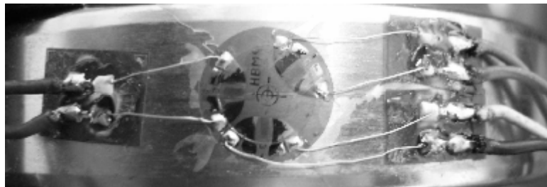
Fig. 5. The electrical connection of the tensiometrical stamp
