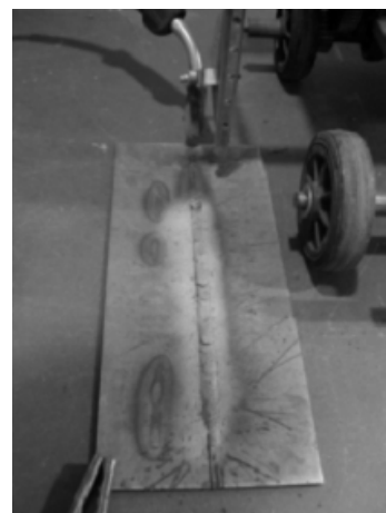
Fig.4. The welding process for arch submerged
