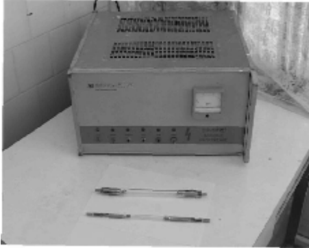
Fig. 2. The condensers block and the optical radiation lamps
